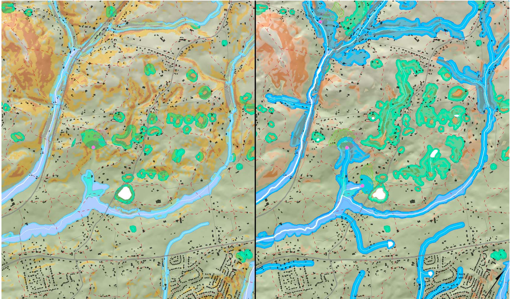
Figure 6.2 Comparison of the BCWGIP buffers (on the left) with the new model results (on the right) in Zone 2. Both buffer methods include the use of the 500-year floodplain in Zone 2, adding 50 feet to its extent. Other features are buffered similarly, with the exception of the use of stream order. In the BCWGIP buffers, 3 rd order or higher streams were buffered more than 2 nd order or lower streams (75 feet vs. 50 feet). In the new model, these values are reversed in order to add more protected land for infiltration and filtering of pollutants in the headwater streams, improving their ability to handle a surge during a flood event. Also, note the improved spring catchments on the right map, used to clip the spring buffers to their overland catchments.
